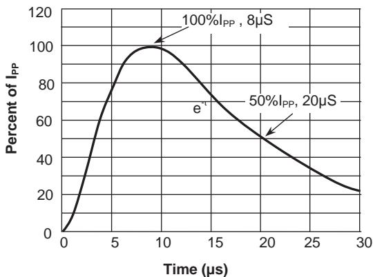
**Fig.4 Pulse Waveform-ESD(IEC61000-4-2)**
